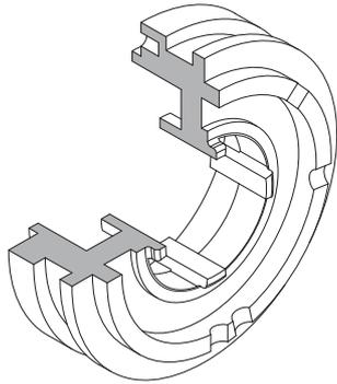
**DSR/F: Roller phase torque limiter, synchronised connection between input and output.**
