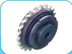
Sliding Safety coupling where the transmission component is fitted between two friction rings and slides when the calibrated torque is reached. The minimum required to have a low cost protection.
