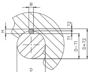
Bore and Keyways according to UNI 6604 (DIN 6885-1)
