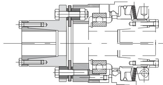
Model **DSS/SG/RF** with single flexing disc coupling **GTR/S**,
