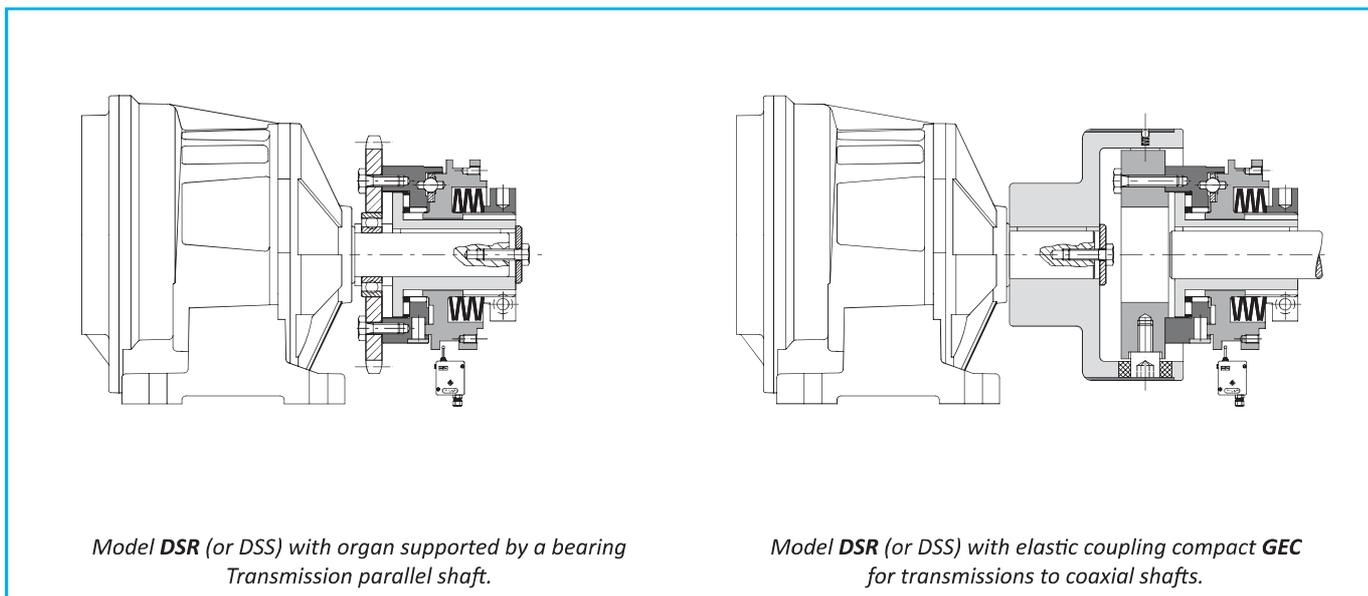
Model **DSR** (or **DSS**) with organ supported by a bearing
