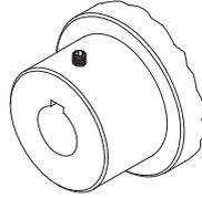
Standard solution on the hubs shown in the catalogue for horizontal assembling.
