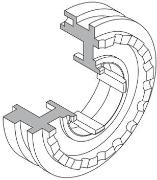
**DSR: Roller torque limiter for steady transmission with high torques and vibrations**
