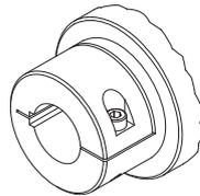
Reduction of angular backlash, during reversing drives, and high torques.
