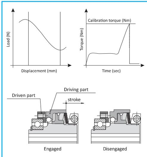
This model of torque limiter negative version to incorporate the following features:
