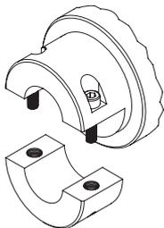
Reduction of angular backlash, and simple radial assembly/disassembly.
