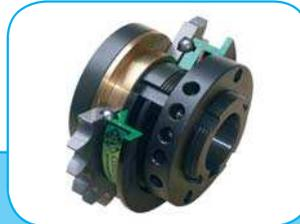
Safety coupling with simple and compact balls inserted directly in the drive element of transmission. The disengagement occurs quickly and safely if the calibrated torque is exceeded.
