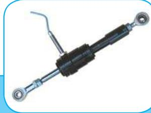
Safety coupling with linear limitation of force. The axial disengagement can take place in both compression and tension once the calibrated force is reached, the re-engagement is automatic.
