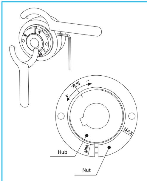
Adjustment of the Negative version is opposite to all other units in our range. Unlike the traditional units, by rotating the adjuster nut clockwise the disengagement torque will reduce, and therefore to increase the torque the nut must be rotated anti-clockwise. To assist the operator in setting, there are clear markings on the nut showing 75% of the max torque and +/- Min/Max directions indicated.
