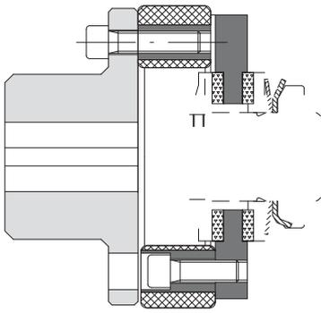
Model **DF** suitable for connections **GF** to coaxial shafts capable of recovering high misalignments.
