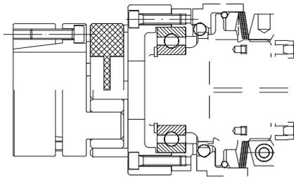
Model **DSS/SG/RF** with backlash free jaw elastic coupling
