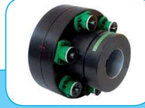
Modular Safety coupling, robust, suitable for "heavy industries" even at high speeds. After disconnection there is free rotation without residual torque, re-engagement is simple and manual.
