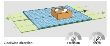
To get a **dynamic rotation to the right**, the two directional belts must run like the picture.
