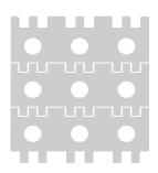
The **small pitch** between the spheres (diameter 12,7 mm and pitch 25,4 mm) allows every type of good transfer and is ideal for small and light packages, unlike traditional roller conveyors.
