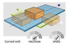
To get a straight exit without loosing relatively too much time, the **directional belt can be activated** also **when the 553 FlexTop is running, while is reducing speed**. The combination of the two speeds will determine the exit curve dimension.
