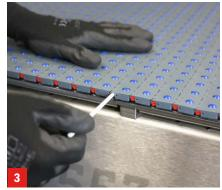
Once the white rod is removed, the belt can be opened easily.
