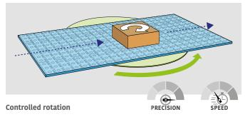
To get a controlled roation, the rotating plate must be activated **when 553** FlexTop is not running.
