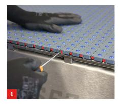
Insert a flat screw driver into the red clip mounted at the sides of the belt, turn it by 90° to leave it from the clip fixation and remove it.
