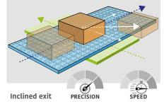
To get a 45° inclined direction, the **speed of the directional belt must be the same** as the speed of the 553 FlexTop and they have to work contemporary.
