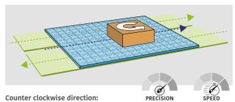
To get a **dynamic rotation to the left**, the two directional belts must run like the picture.
