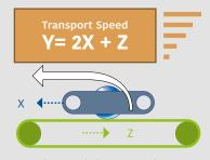
553 FlexTop belt mounted over a longitudinal conveyor running in opposite direction.
