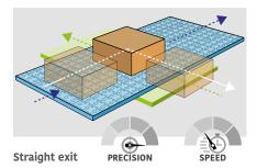
To get a completely straight exit, **the directional belt must be activated when 553 FlexTop is not running**.
