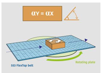
**553 FlexTop belt with a 360° rotating plate underneath** Useful option used to easily positioning the good.
