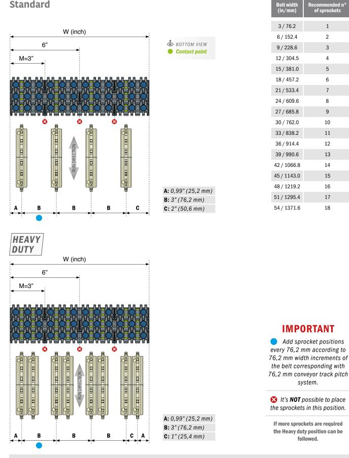
HEAVY DUTY position is ideal in case the load of the application is close to the belt limit or in case there is an high number of starts/stops during production.
