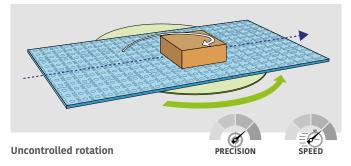
If the rotating plate get activated while the modular belt is running, the **good will rotate in more space.**
