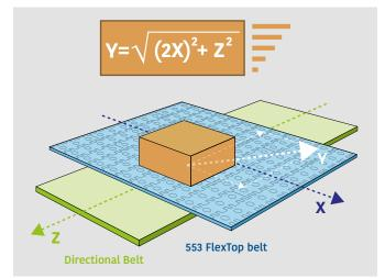
**553 FlexTop belt with directional belt mounted perpendicularly** The difference in speed between the 553 FlexTop belt and the directional belt determines the direction angle of the good.
