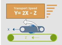
553 FlexTop belt mounted over a longitudinal conveyor running in the same direction.
