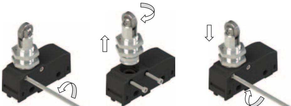
Thanks to the new patented lateral fixing system, it's possible to rotate the roller of microswitches MK ●●●15 and MK ●●●17 in 90° steps.
